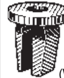
14755 (379830-S) White Nylon 3/8" Wide, 3/8" Long #8 Screw Size Fits Into 1/4" Sq. Hole Ford 1986-On UNIT PACKAGE: 25
